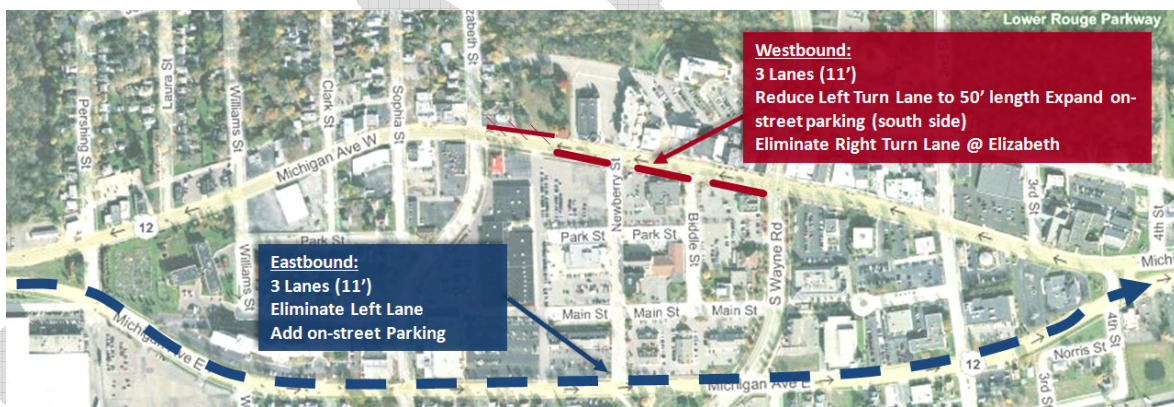
Current and projected traffic volumes along Michigan Avenue should be handled effectively with 3 lanes in each direction.
