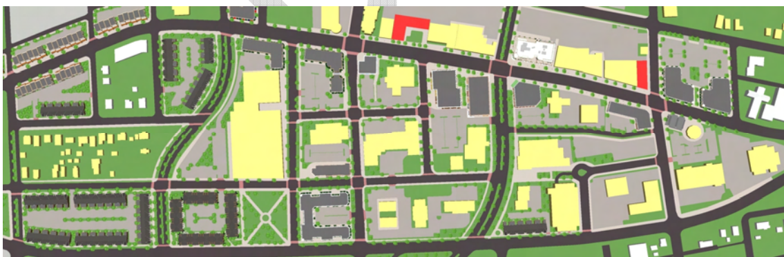
A preliminary 3-d model was prepared to visualize many of the initial concepts (yellow buildings are current buildings to remain, dark grey and red are sites/buildings for potential redevelopment).
